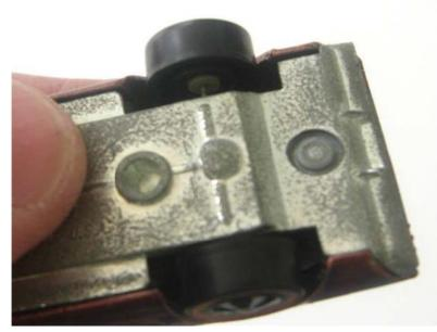
Support one side of the wheel with your thumb as you hold the car. Slide the wrench into position as shown. While you are supporting the wheel with your thumb, begin to pry the wheel off slowly and gently. Make sure you are not pushing against the bearing with the wrench. All the force should be on the backside of the wheel, not the bearing. Your thumb will hold the wheel straight so the wheel does not twist while you are prying with the wrench on the opposite side of the wheel.
